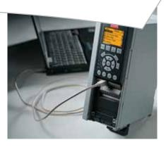
The VLT® HVAC Drive can be remote commissioned and monitored through a USB pluggable cable or BMS network communications. VLT® Set up Software MCT 10 and Language Changer make drive operation child's play.
